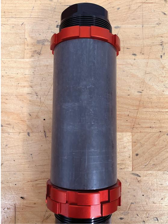
Figure 5: Use all 3 lock rings per 1 bump stop
