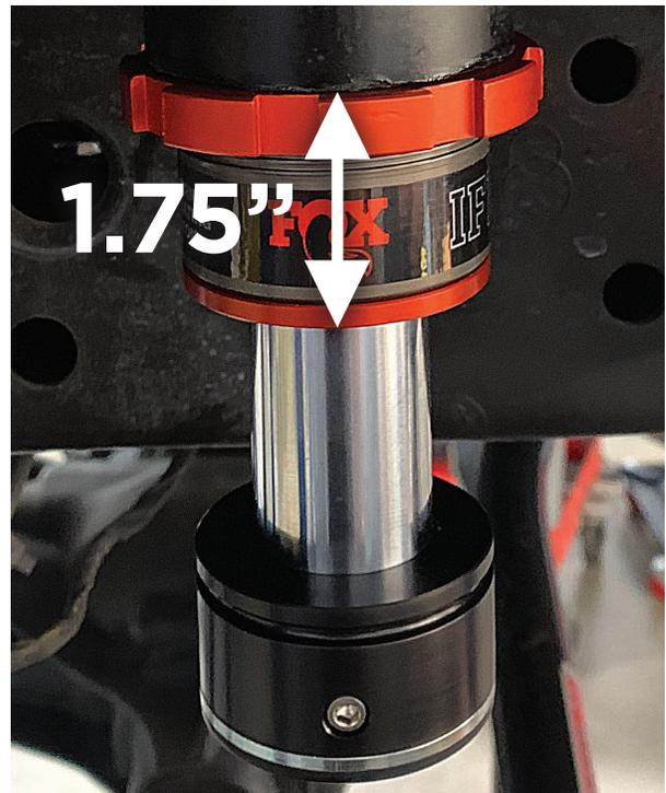
11. Apply medium strength thread locker to the lock rings and Use all 3 lock rings per 1 bump stop. Tighten both the upper and lower lock rings using supplied spanner wrench and use the flat side of the 3rd lock ring to us as a jam nut against the lower lock ring (Figure 5).
