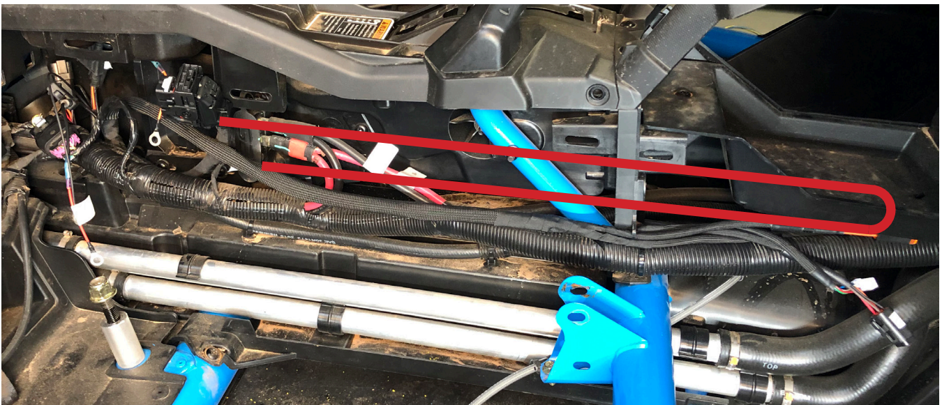
Figure 11b: Shows how to consume excess wire length on 2-seat models.
