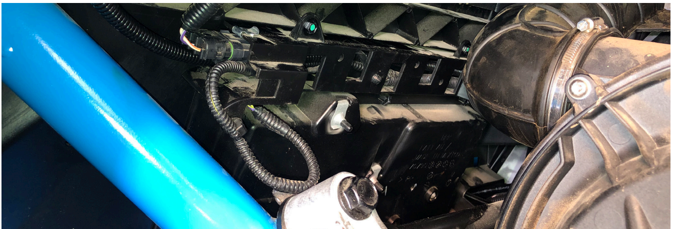
Figure 9c: Shows cable channel installed with the left-side rear shock lead.
