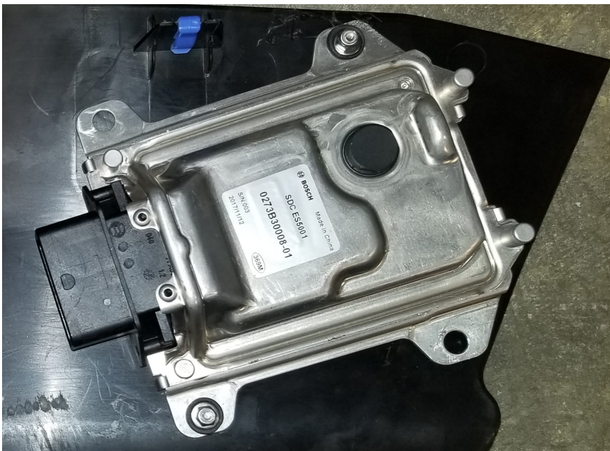
Figure 15b: Shows the ECU installed to the panel with the supplied rubber grommets and M4 mounting hardware.
