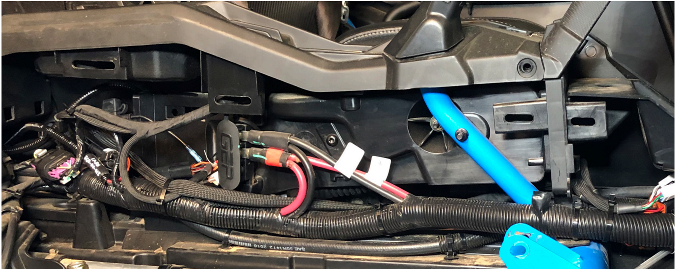
Figure 14a: Shows a secured portion of the main harness towards the rear of the center console. Note the loop created with the first 16 inches of the harness.
