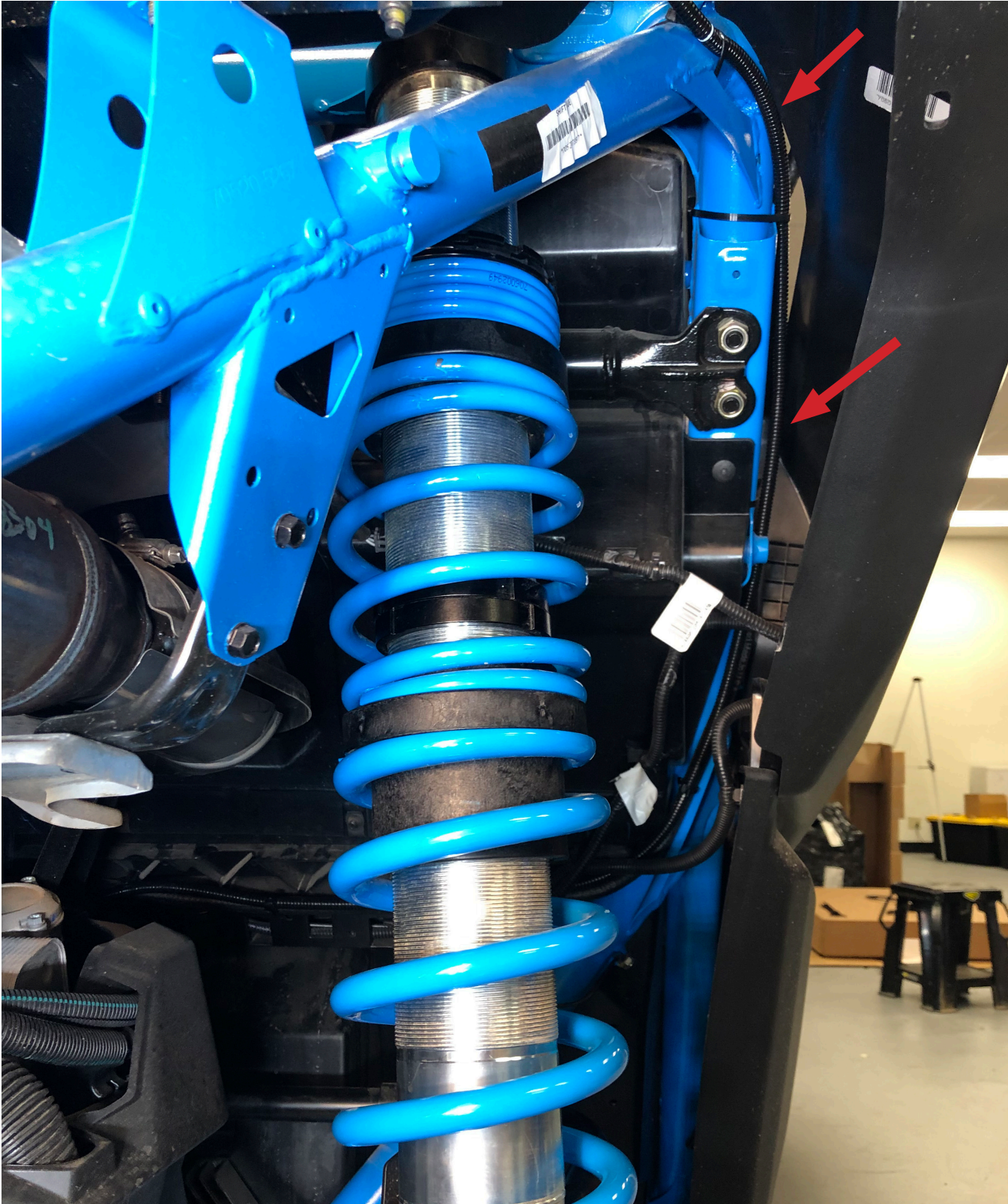
Figure 10: Shows harness routing along the back of the right-side frame rails before reaching the OEM harness bundle.
