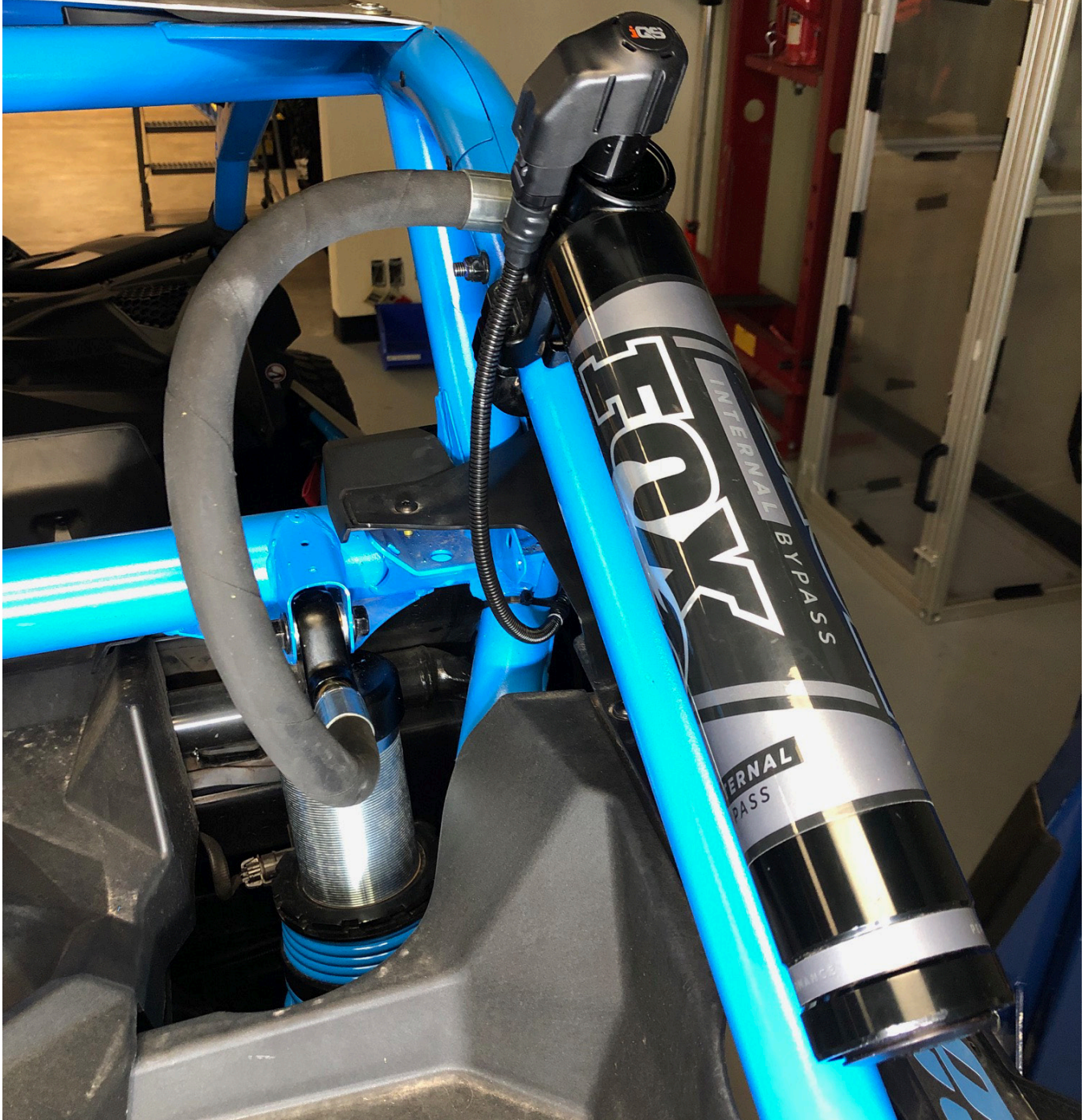
Figure 1a: Shows proper rear shock orientation with iQS connector facing toward the center of the vehicle.
