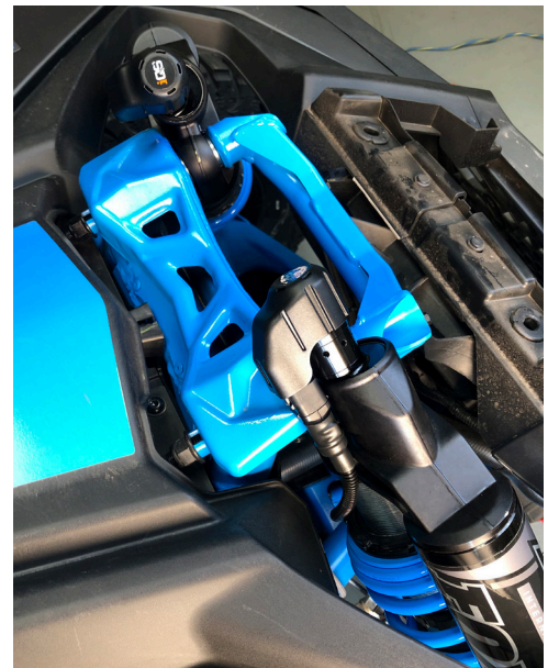
Figure 4c: iQS motor connection facing rearward with leads passing under upper shock mounting bolt.
