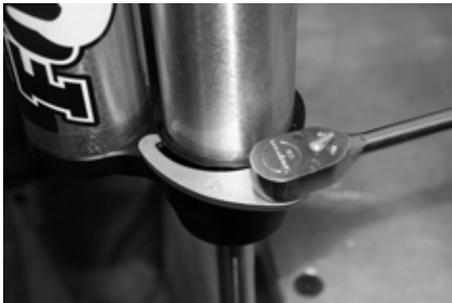
Fig. 7: Spanner wrench loosen
