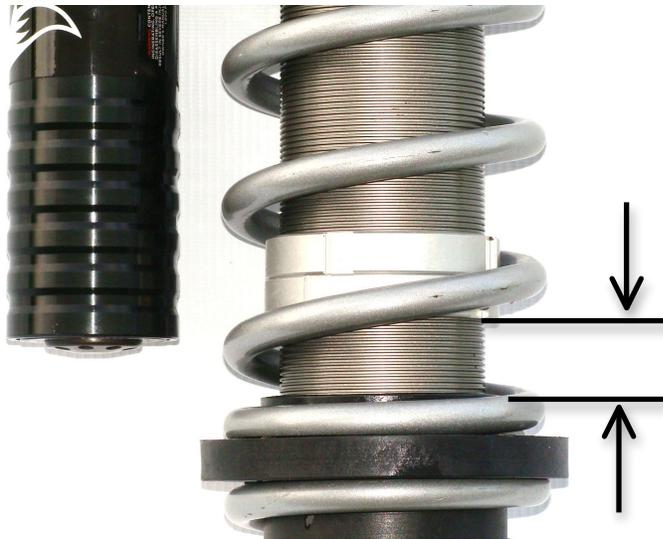
Crossover ring placement value should match the distance from the top of the spring coupler to the bottom of the crossover ring. Example .912 inches
