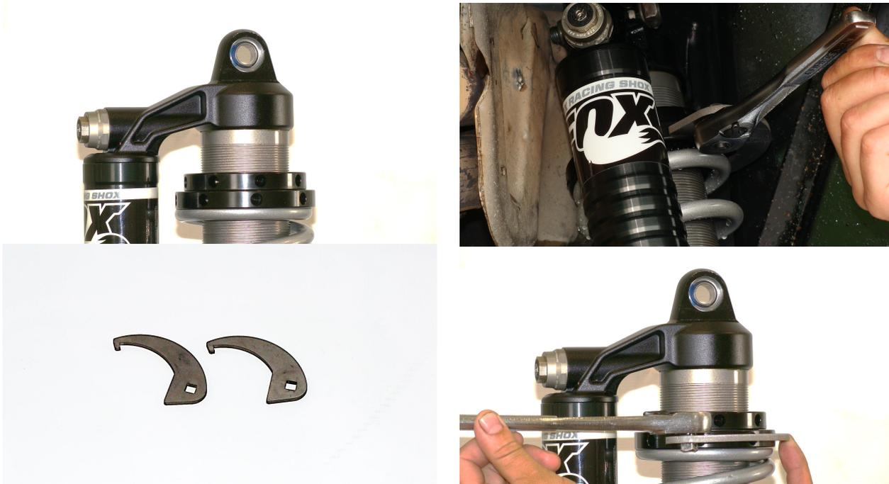
P/N 398-00-393 Tooling: Spanner, Preload Wrench
