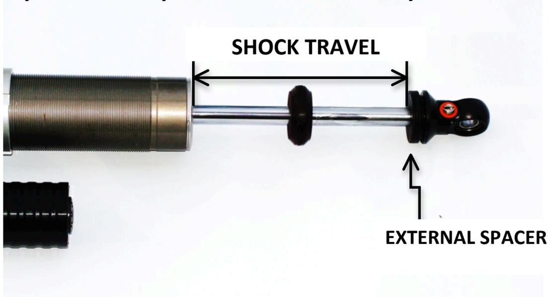
SOME SHOCKS USE EXTERNAL SPACERS BELOW THE BUMP STOP TO LIMIT TRAVEL. DO NOT INCLUDE THE SPACER LENGTH AS PART OF THE TRAVEL.
