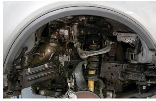
Fig. 1: Pull the fender liner.
