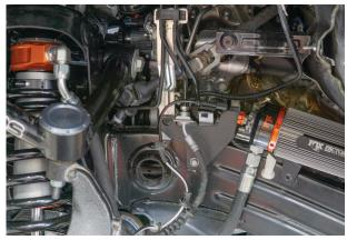
Fig. 25: Mount the reservoir bracket.
