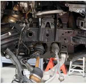
Fig. 10: Free the coil-over from the coil bucket.
