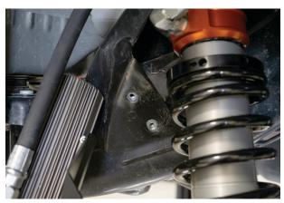
Fig. 41: Align backing plate with the frame.
