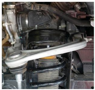
Fig. 7: DO NOT remove the center nut.
