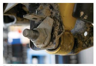
Fig. 31: Loosen the lower mounting bolt.
