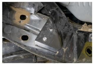
Fig. 40: Locate the backing plate's speed nuts with the holes in the frame.
