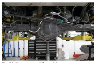
Fig. 30: Support the differential.
