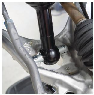
Fig. 13: Fasten the bar-pin bolts.
