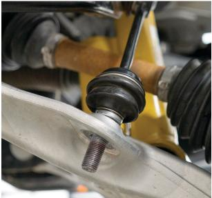
Fig. 4: Disconnect sway bar end link.
