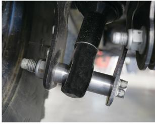
Fig. 36: Note the larger spacer is on the inboard side.
