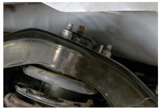
Fig. 32: Do not remove the center nut.
