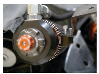
Fig. 37: Mount the reservoir bracket.
