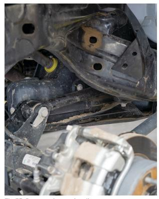
Fig.33: Remove the stock coil-over.
