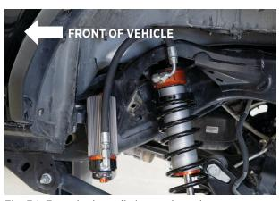
Fig. 34: Face the hose fitting outboard.
