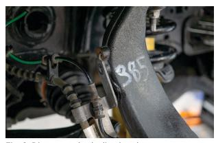
Fig. 2: Disconnect brake line bracket.
