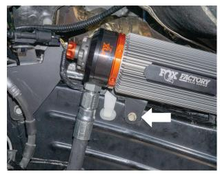
Fig. 27: Install the self-tapping screw.
