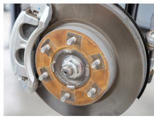
Fig. 15: Fasten the axle nut.
