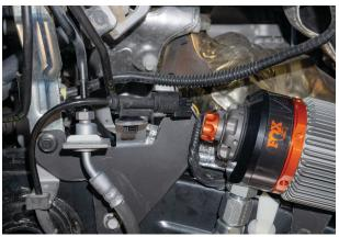
Fig. 26: Fish the ABS wire through the bracket.
