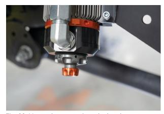
Fig. 22: Mount the reservoir to the bracket.
