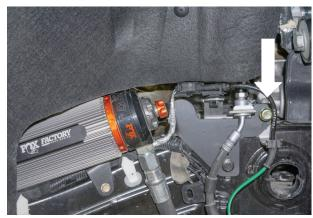
Fig. 24: Install the provided bolt on the passenger side's reservoir bracket.
