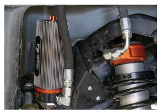
Fig. 42: Mount the reservoir bracket.
