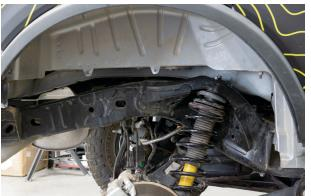
Fig. 29: Pull the fender liner.
