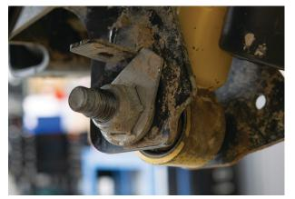
Fig. 26: Loosen the lower mounting bolt.
