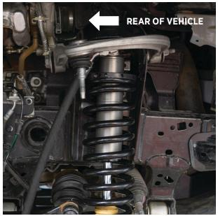
Fig. 13: Install the FOX coil-over.
