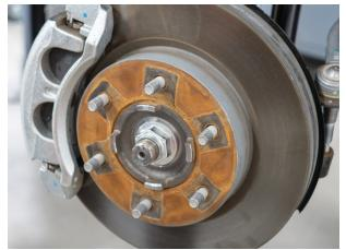
Fig. 18: Fasten the axle nut.
