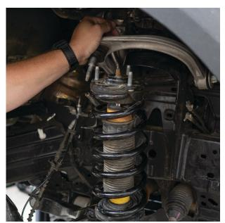
Fig. 10: Free the coil-over from the coil bucket.
