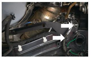
Fig. 3: Mount the reservoir bracket.
