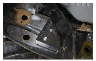
Fig. 30: Align backing plate with the frame.
