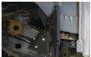
Fig. 31: Mount the reservoir bracket.
