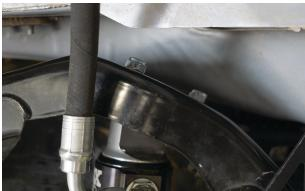
Fig. 32: Face the hose fitting outboard.
