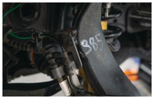
Fig. 4: Disconnect brake line bracket.
