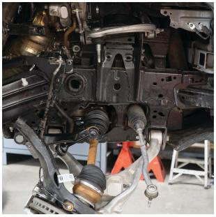
Fig. 12: Free the coil-over from the coil bucket.
