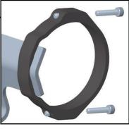
Fig. 16a: Diagram of reservoir and bracket interface.
