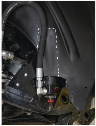
Fig. 36: Test fit the fender liner.
