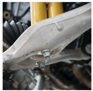
Fig. 11: Take off the bar-pin bolts.
