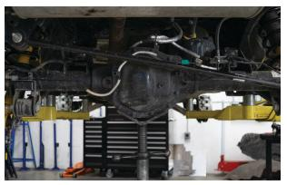
Fig. 25: Support the differential.
