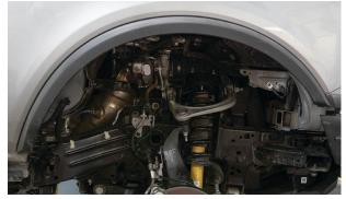
Fig. 1: Pull the fender liner.
