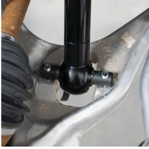
Fig. 15: Fasten the bar-pin bolts.
