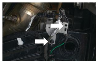
Fig. 2: Remove the brake line bracket bolts.
