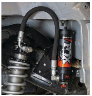
Fig. 34: Mount the reservoir to the mounting bracket.
