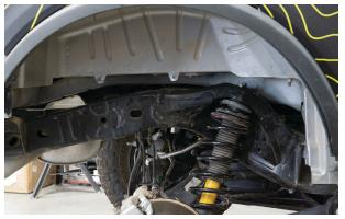
Fig. 24: Pull the fender liner.
