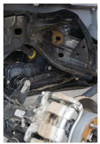
6. Remove the top hat nuts first, then the lower shock mount bolt. Slide the stock coil-over out (Fig. 28).
