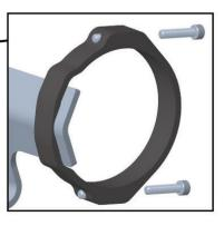
Fig. 9a: Mount the reservoir flush to the bracket.
