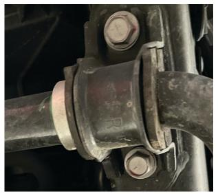
Fig. 3a: Remove sway bar bolts.
