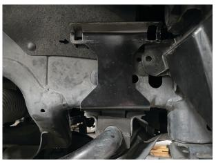
Fig. 8: Install the reservior bracket.
