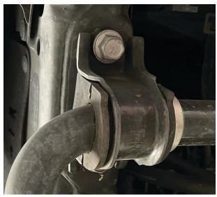
Fig. 3b: Remove sway bar bolts.
