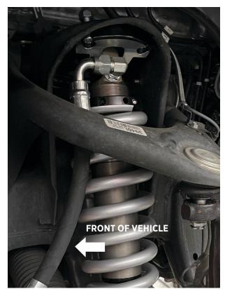
Fig. 7b: Machined flat on top hat. Fig. 7a: Install FOX shock assembly.
