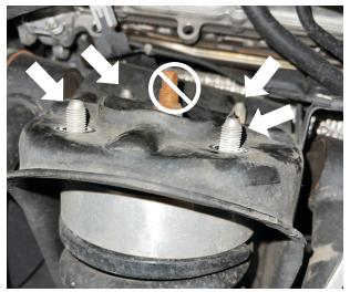
Fig. 4: Remove top hat nuts.
