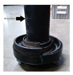
Figure 6: Top-mount and dust cover for removal
