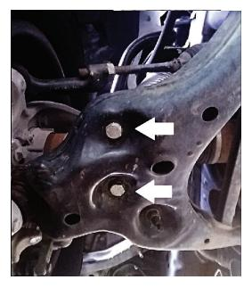
Figure 4: Bolt location for connection between lower shock and lower control arm
