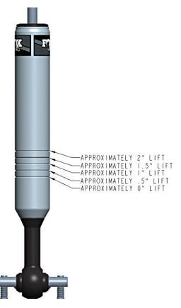
Figure 7: Illustration of groove/lift height options
