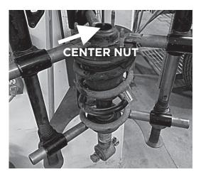
Figure 5: Professional spring removal tool
