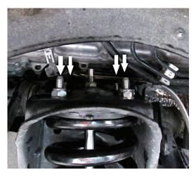
Figure 3: Top mount fastening to frame
