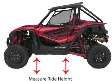
at each end of flat section of the frame.
