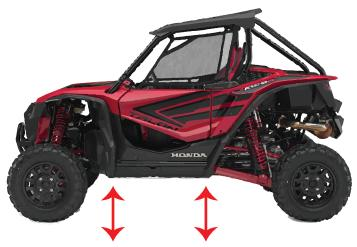
Measure Ride Height at each end of flat section of the frame.
