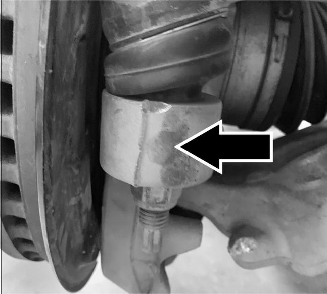
**Note:** Once the nut is removed use a mallet and strike the knuckle in the above highlighted area to allow the tie rod to un-index itself.
