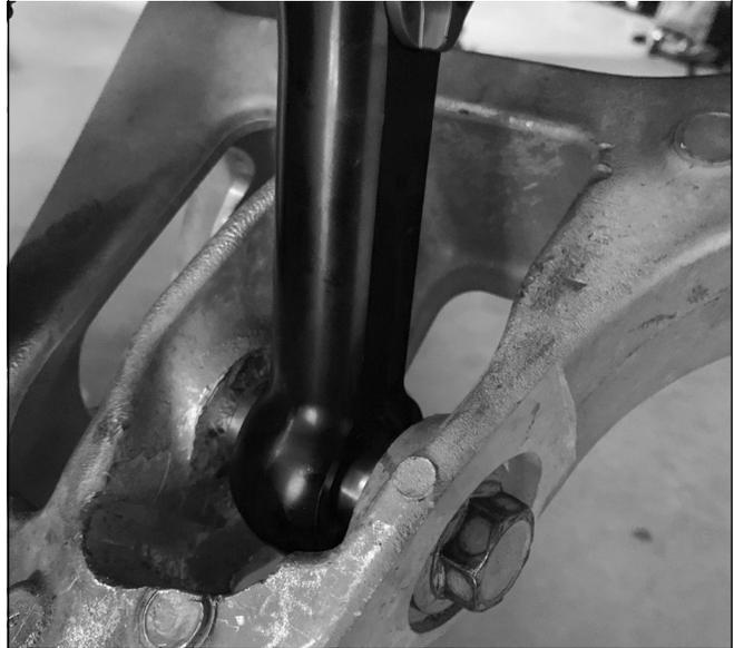
**Note: The user can clock the eyelet with the switch facing away or towards the front of the truck. Rotate the eyelet to have the switch face the back of the truck if desired.**
