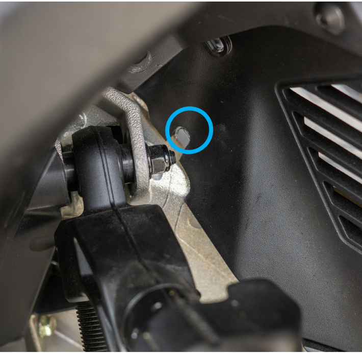
Figure 15: 3/8 inch hole and slot along edge of panel
