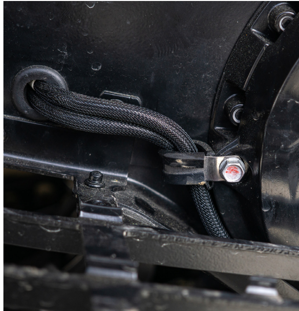
Figure 5: Final hole and grommet placement
