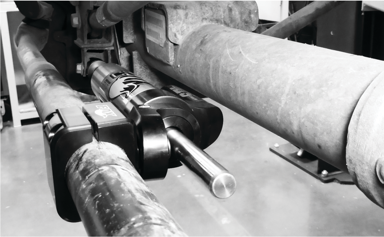
Fig. 2: Loosely mount the stabilizer to the track bar.
