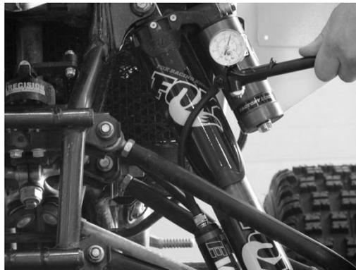
**STEP 2** Thread the pump onto the EVOL air filler valve until it is fully seated and air pressure registers on the pumps high pressure scale.
