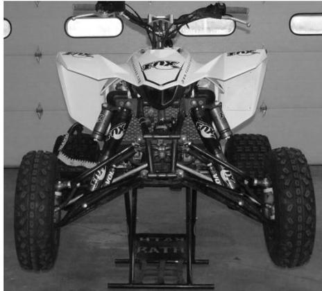
**STEP 1** Ensure that your ATV is safely supported on a stand with the front wheels off the ground and the suspension fully extended.
